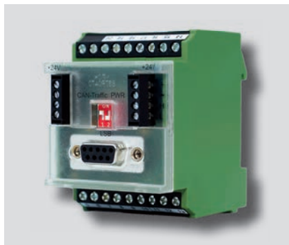
LEM100 expansion module for LSB 667R0400-1
