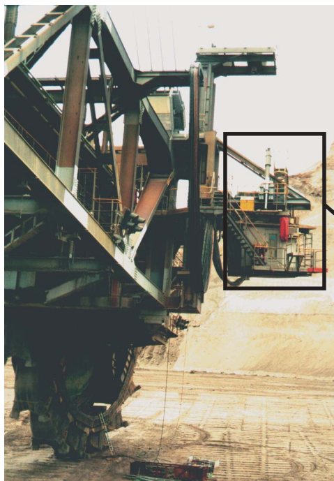
Cab level regulation open-pit lignite mine
